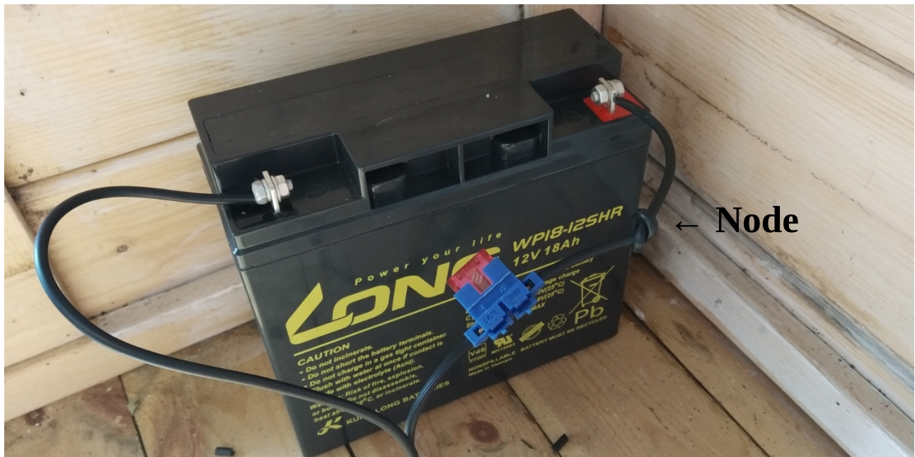
AGM 12 Volt battery with circuit breaker (blue) with fuse (red). Since both wires are black, the positive wire is marked with a node.
